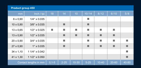
Quality band saw blade with particularly wear-resistant, high cutting accuracy in a wide variation of dimensions and toothings with neutral rake angle.
